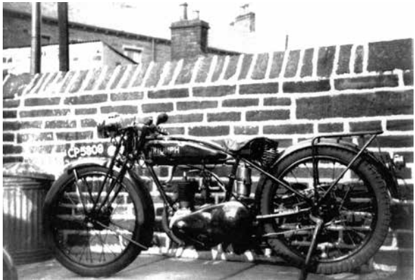
1927 Triumph 277cc motor cycle with acetylene gas lighting
